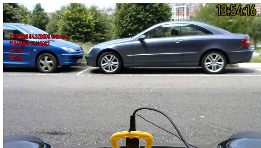
Figure 10. On-screen display of radar data. Distance and type of objects.
