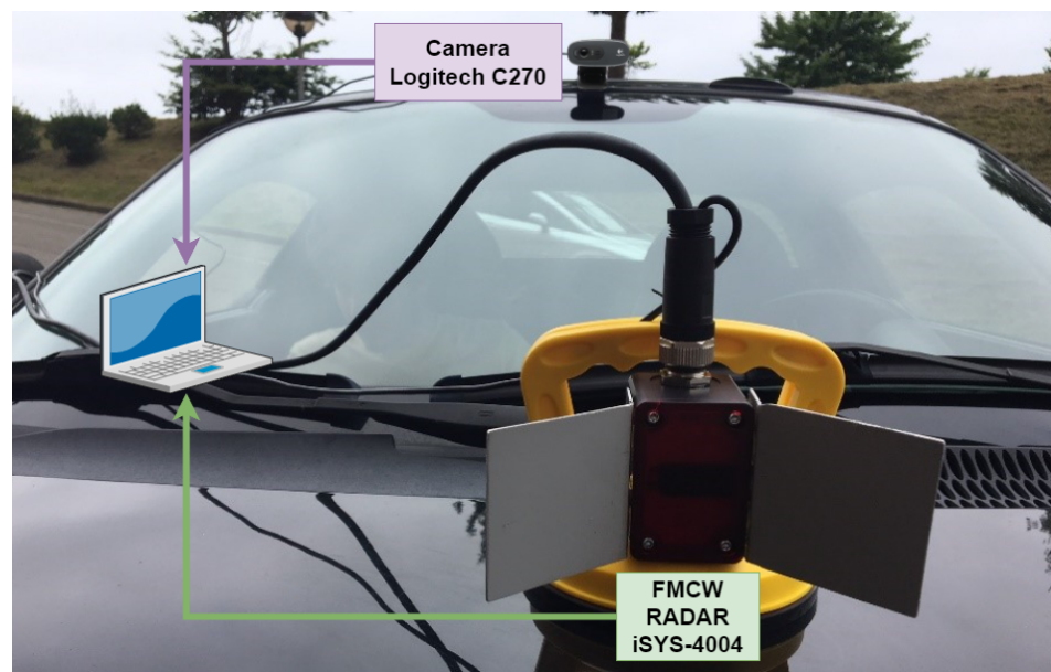
Figure 5. Mounting of the radar on the vehicle.
