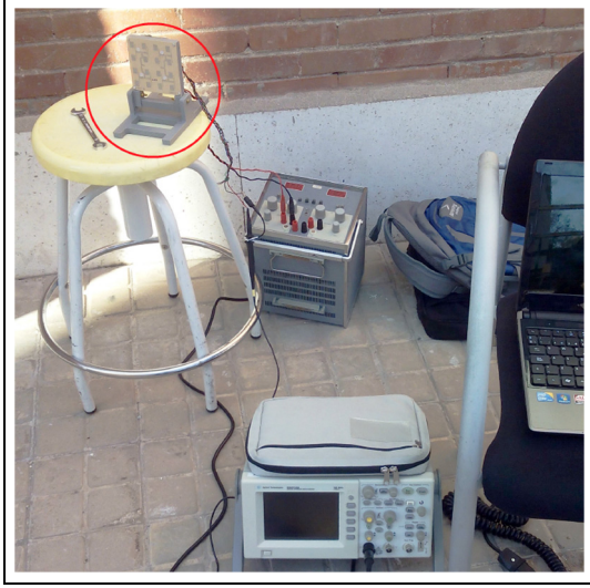
Figure 3. Deployment of a radar for measuring. The low-cost radar is inside the circle.
