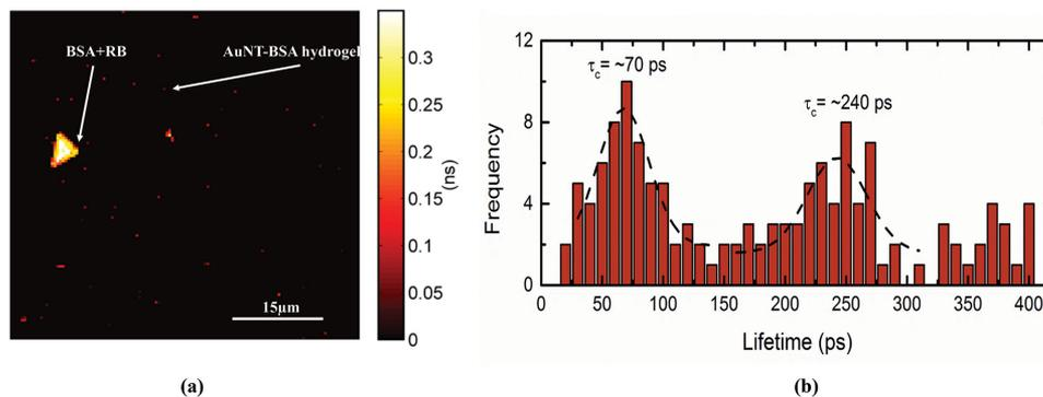
**Figure 6.** FLIM of the AuNT-BSA hydrogel nanoparticles fabricated using 2 mW incident laser. a) FLIM image showing the control BSA hydrogel and AuNT-BSA hydrogel in the same FOV. b) Histogram of lifetimes obtained from the same FOV indicating two separate lifetimes of  $\approx 70$  and  $\approx 240$  ps for AuNT-BSA hydrogel and control BSA hydrogel, respectively.
