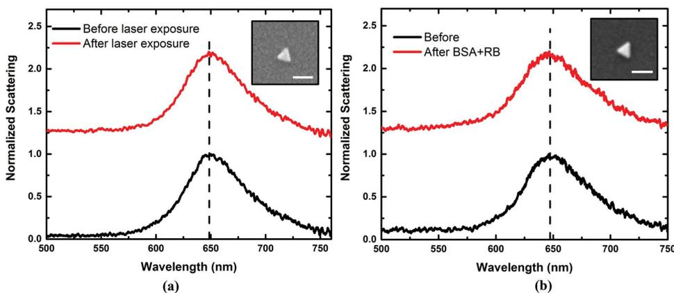
**Figure 5.** Dark-field scattering spectra of two independent controls: a) Before and after 2 mW laser irradiation without the presence of BSA and RB and b) before and after exposure of AuNT to BSA and RB fabrication solution without any laser irradiation. The “after” plot was offset along the  $y$ -axis for clarity. The inset shows the corresponding high-magnification SEM image, with a scale bar of 100 nm.
