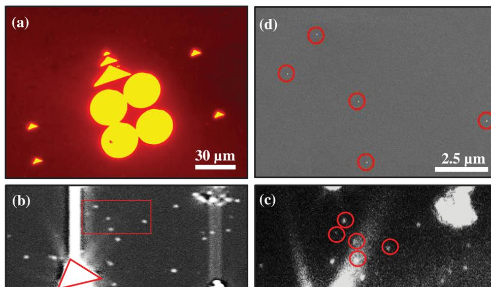
**Figure 3.** Correlated single-particle dark-field spectroscopy and SEM. a) Typical markers of BSA hydrogel prepared by direct laser writing to localize the individual AuNTs. b) Dark-field image of multiple nanoparticles in the vicinity of the marker before fabrication. The extremely bright spot is the strong scattering from the marker. c) Dark-field image of the same region after fabrication. d) SEM imaging of the region indicating the presence of well-separated single nanoparticles.
