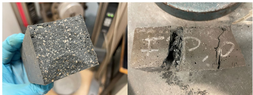
Fig. 4 Prismatic samples after flexural test (left) and compression test (right). Mortar with PP fibers
