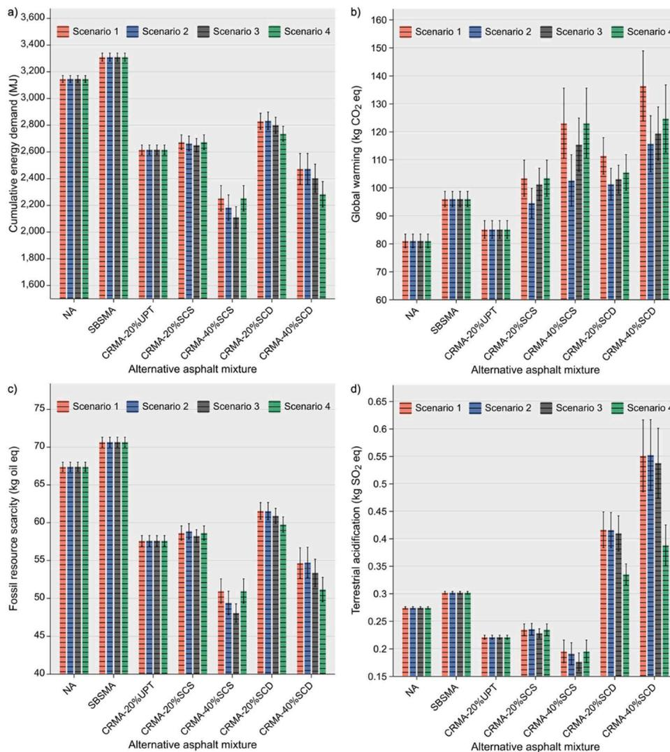
**Fig. 13.** Comparative environmental impact results of scale-up scenarios: (a) CED, (b) GW, (c) FRS, (d) TA.
