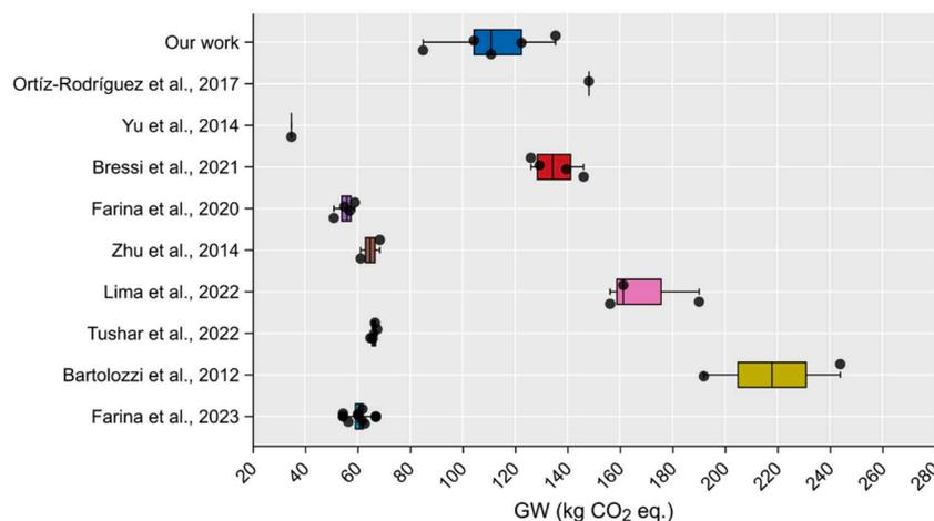
Fig. 4. Environmental impact (global warming) comparison of valorizing ELTs in asphalt mixtures between our study and other relevant studies (Bartolozzi et al., 2012; Bressi et al., 2021; Farina et al., 2023, 2014; Ortiz-Rodríguez et al., 2017; Siverio Lima et al., 2022; Tushar et al., 2022; Yu et al., 2014; Zhu et al., 2014).
