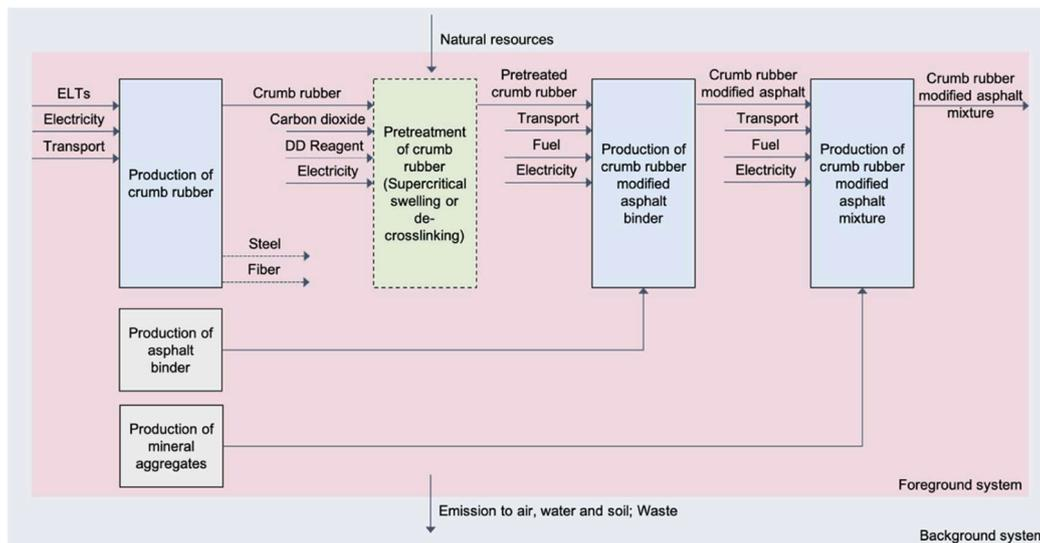
Fig. 1. System boundary of CRMA (with/without supercritical pretreatments of CR).
