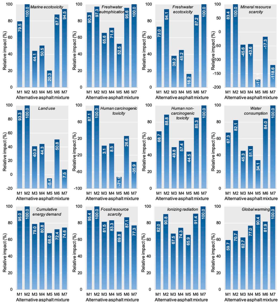
Fig. 2. Relative impact scores of midpoint indicators for different alternative asphalt mixtures. Key: M1 = NA; M2 = SBSMA; M3 = CRMA-20 %UPT; M4 = CRMA-20 %SCS; M5 = CRMA-40 %SCS; M6 = CRMA-20 %SCD; M7 = CRMA-40 %SCD.
