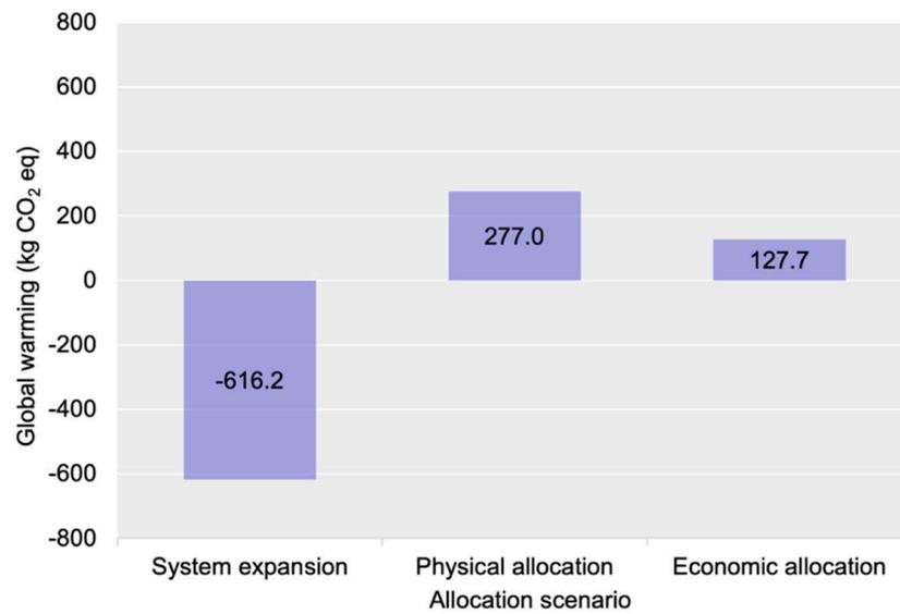
Fig. 7. Scenario analysis on producing 1 ton of CR considering different allocation scenarios.
