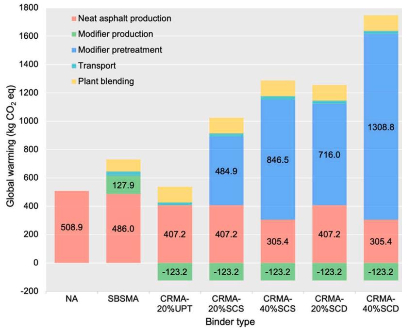
Fig. 6. Process contribution to environmental impacts of producing 1 ton of asphalt binder.
