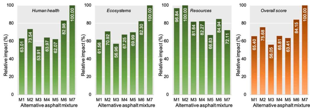
Fig. 3. Relative impact scores of endpoint indicators and overall score for different alternative asphalt mixtures. Key: M1 = NA; M2 = SBSMA; M3 = CRMA-20 %UPT; M4 = CRMA-20 %SCS; M5 = CRMA-40 %SCS; M6 = CRMA-20 %SCD; M7 = CRMA-40 %SCD.
