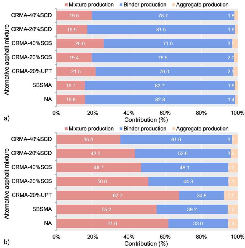
Fig. 5. Process contribution to the overall environmental impacts of producing 1 ton of asphalt mixture: (a) Cumulative energy demand; (b) Global warming.
