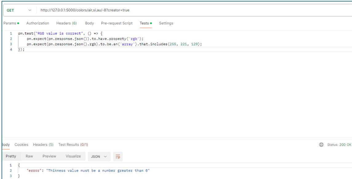
The screenshot shows a REST client interface with a GET request to `http://127.0.0.1:5000/colors/air,si,au/-8?creator=true`. The Tests tab is active, displaying the following test script:
