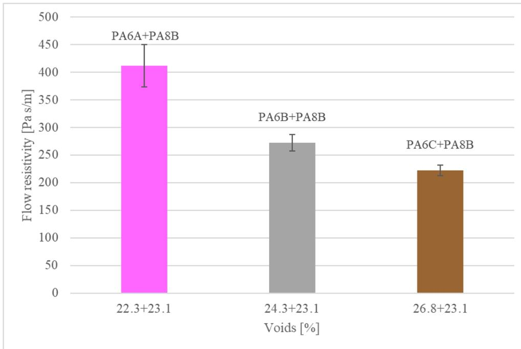
Figure 13. Flow resistivity of 2LPA specimens with different void content of the top layer.
