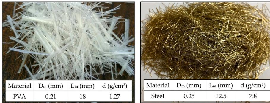
Fig. 1. Appearance and characteristics of the fibers used.
