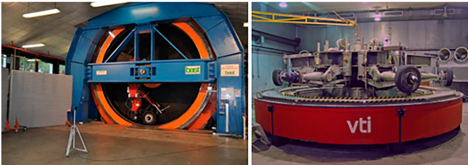
Figure 6. Left: vertical drums from BAST; right, VTI's road simulator (Andersson-Sköld et al., 2020).
