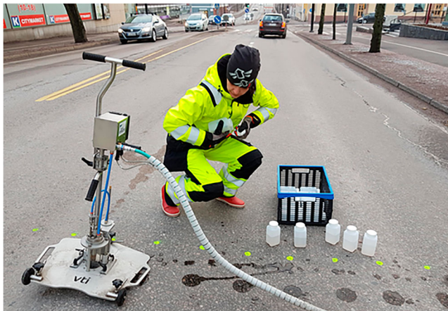
Figure 7. Sampling in a city street with WDS. Picture: Roosa Ritola (SYKE and SKYE, 2020).
