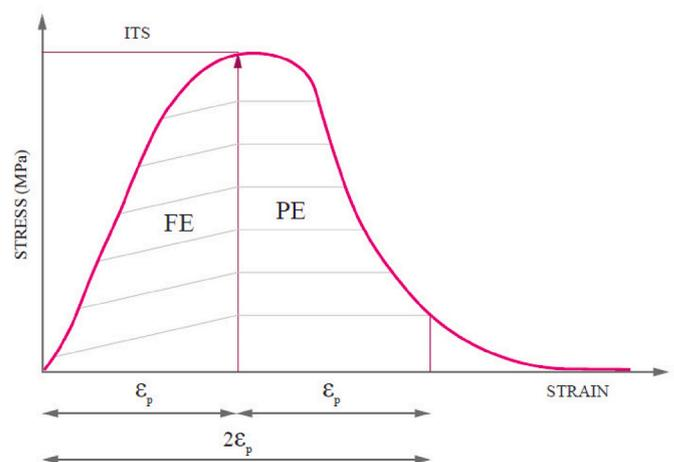
Fig. 4. Stress-strain curve recorded from ITS.
