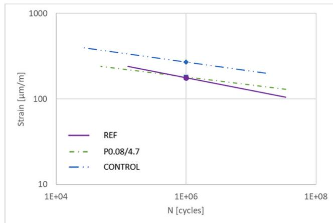
**Fig. 9.** Fatigue test results of the final designs.
