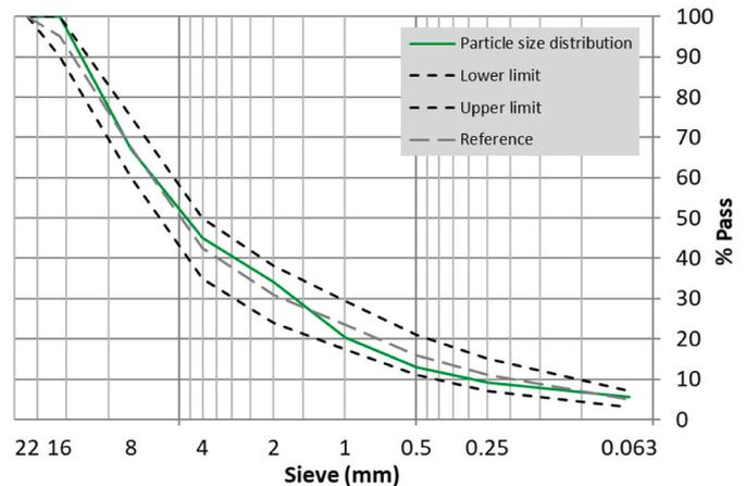
Fig. 1. Particle size distribution of the mixtures.
