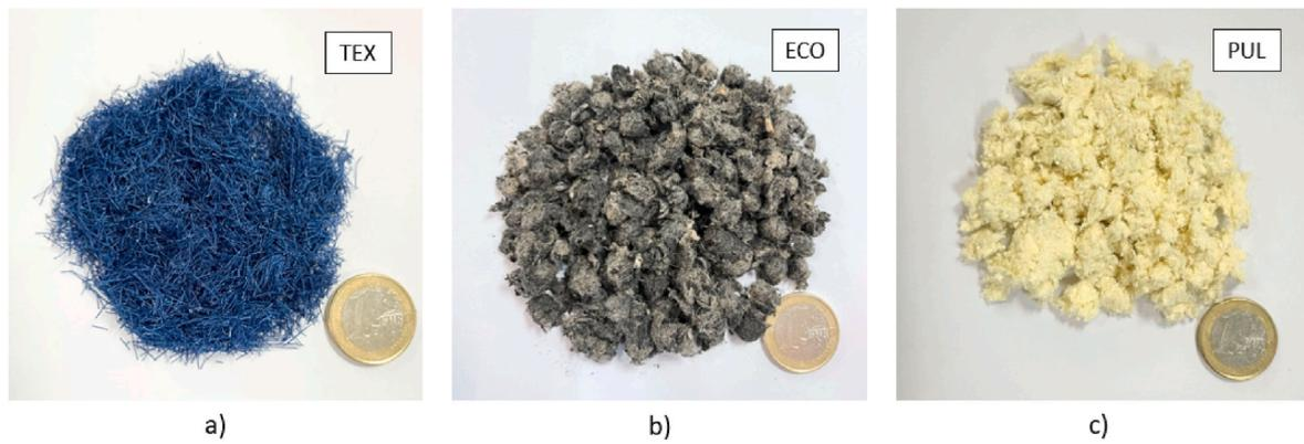
Fig. 2. Fibres used in the study: (a) Textil (TEX); (b) Ecofibra (ECO); (c) Aramid pulp (PUL).
