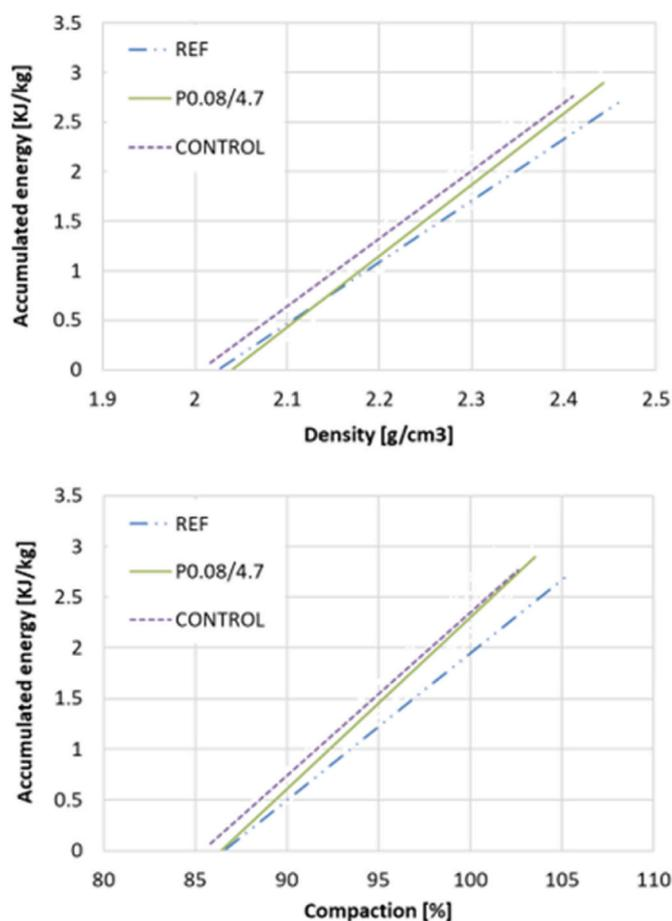
Fig. 8. Compaction energy of the final mixtures.
