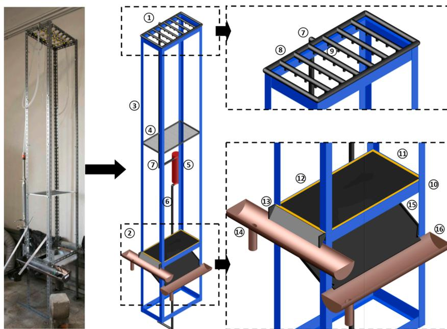
**Figure 2.** Rainfall simulator photograph and details. 1: Raindrops maker; 2: Testing area; 3: Support structure; 4: Plastic grid; 5: Flowmeter; 6: Flowmeter Inlet pipe; 7: Flowmeter Outlet pipe; 8: Flexible pipes; 9: Drippers; 10: Specimen support; 11: Specimen; 12: Waterproofing; 13: Runoff conveyance ramp; 14: Runoff collecting pipe; 15: Infiltrated water conveyance ramp; 16: Infiltrated water collecting pipe.
