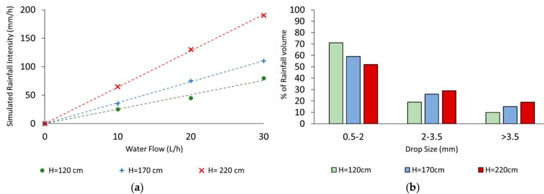
**Figure 3.** Rainfall simulator calibration: (a) rainfall intensity; and (b) drop size distribution.
