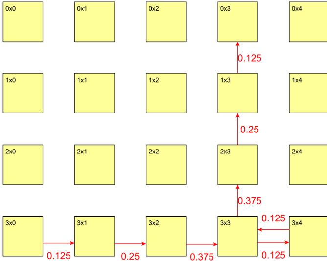
Fig. 9. Accumulated transmission rate of each link of the evaluation system.
