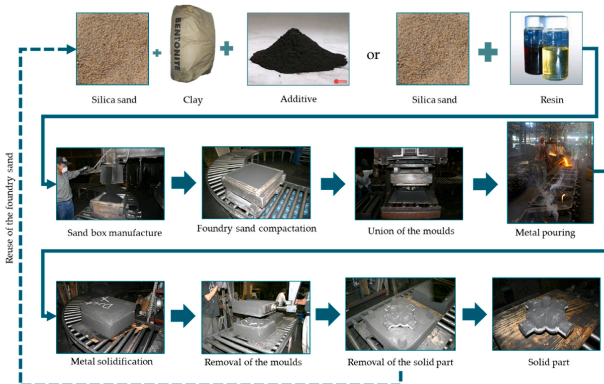
Fig. 1. Metal casting process (images under CC by 3.0).
