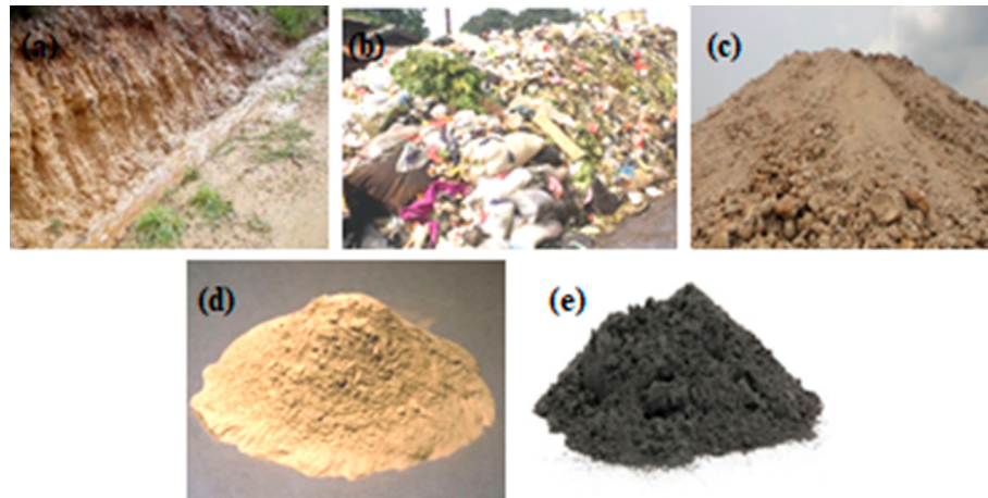
Fig. 3 – The cement raw material before the combustion process to become the cement concentrate: (a) the Mediterranean soil; (b) the household waste; (c) the calcined clay; (d) the pulverized fuel ash; and (e) the bottom ash.
