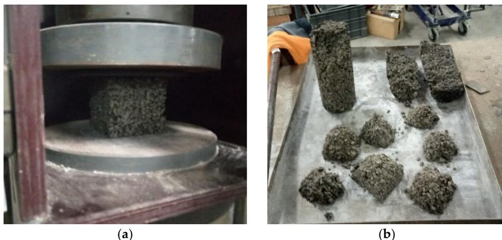
**Figure 3.** Setup demonstrating the compressive test: (a) before crushing; (b) after crushing.
