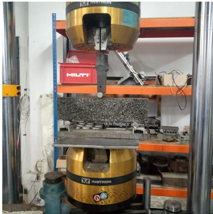
**Figure 5.** Setup demonstrating a specimen subject to the flexural test.
