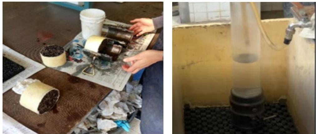
Figure 6. Setup demonstrating the permeability test.
