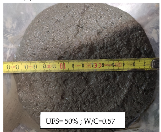
Figure 6. Mortar workability: slump table test results in cm (a) and comparative example for a fixed UFS value (b).
