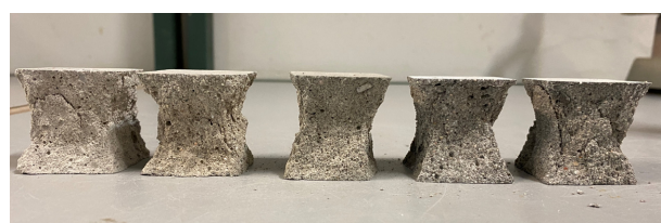
Figure 16. Mortar specimens with UFS, from 0 to 100%.
