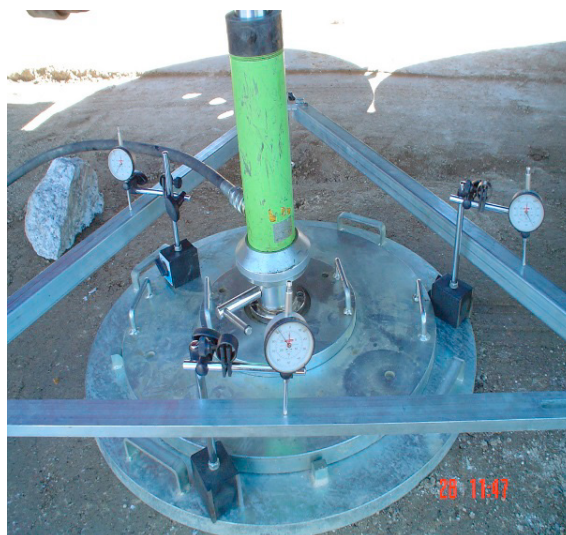
Figure 8. Standard load plates (300, 600 and 762mm)
