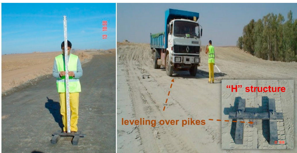
Figure 6. (a) Wheel impression test: leveling over pikes; (b) Schematic diagram of wheel impression test
