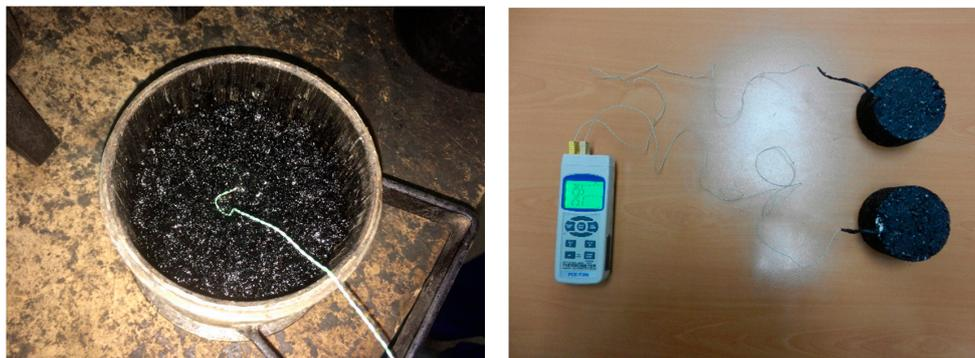
**Figure 1.** Thermo-sensor inside the specimens.
