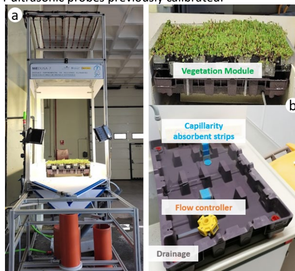
Figure 1 (a) Rainfall simulator and (b) Hydropack © green roof module
