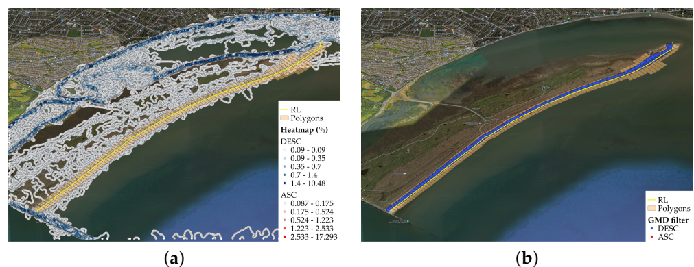
Figure 9. SLs produced for Bull Island including both ASC and DESC tracks (a). Filtering applied to the scene and points selected to produce time series and change rate (b). Source of aerial imagery: Google, ©2023 Maxar Technologies.
