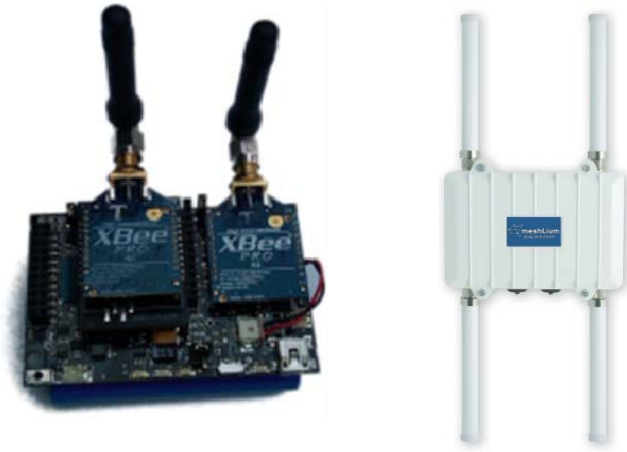
Figure 2. IoT node/repeater (left) and Gateway (right) architecture
