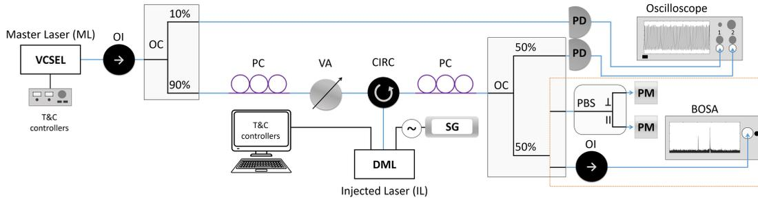
**Fig. 1.** Experimental setup: a VCSEL (Master Laser) provides cw optical injection to a DML (Injected Laser). BOSA: Brillouin Optical Spectrum Analyzer, CIRC: Circulator, T&C: Temperature and Current, OC: Optical Coupler, OI: Optical Isolator, PBS: Polarization Beam Splitter, PC: Polarization Controller, PD: Photo Diode, PM: Power Meter, SG: Signal Generator, VA: Variable Attenuator.
