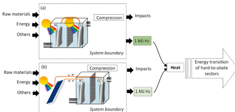
**Fig. 2.** System boundary of H<sub>2</sub> production to provide heat in the energy transition (1 MJ) by: a) unbiased-PEC; and b) PV-WE.
