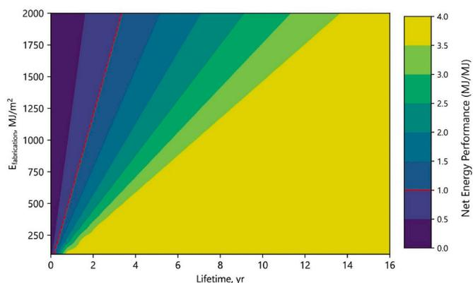
Fig. 3. Sensitivity analysis of the energy input for PEC cell fabrication and lifetime at 10% STH. The red line represents the case when the amount of H<sub>2</sub> energy produced is the same as the one used or embodied in the system for its production. NREL target is adapted from James et al., (2009). (For interpretation of the references to colour in this figure legend, the reader is referred to the Web version of this article.)
