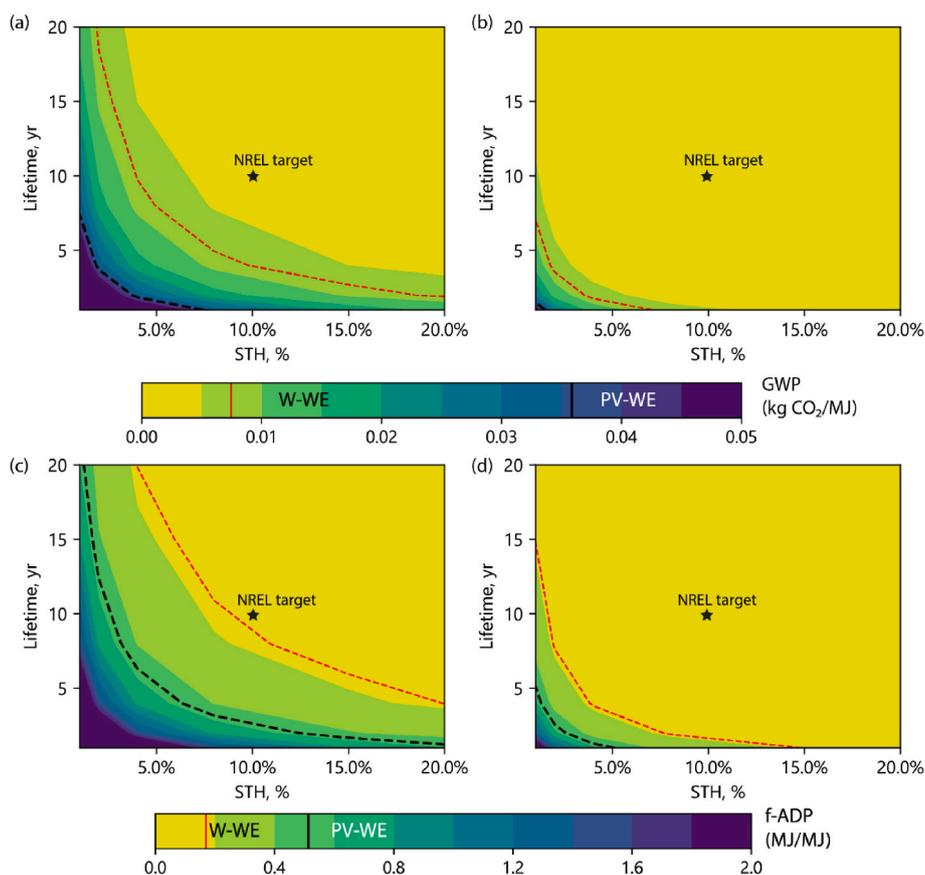
Fig. 4. Results of the bivariate sensitivity assessment in the GWP (a and b) and f-ADP (c and d). The effect of using EU-PV solar is shown in (a) and (c). The effect of using EU-wind electricity is shown in (b) and (d). Reference W-WE and PV-WE are adapted from Rumayor et al. (2022b) and detailed in the Supporting Information. NREL target is adapted from James et al., (2009).
