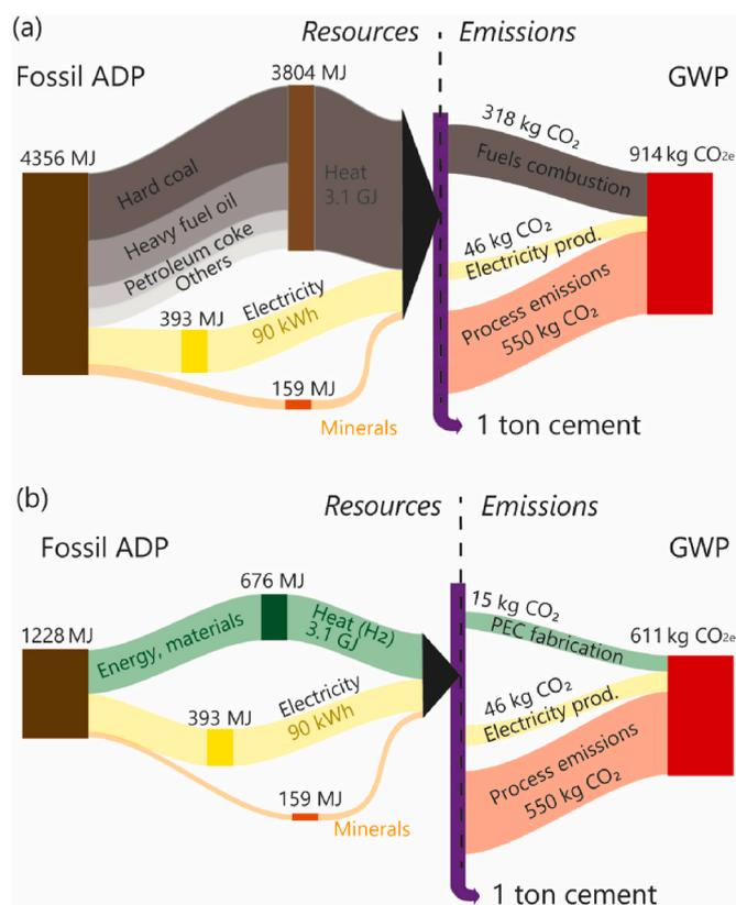
Fig. 5. Example of decarbonization/defossilization synergy of a) conventional cement production; and b) cement production using fuel switching to super-H<sub>2</sub> at the NREL-conditions (10% STH, 7 years lifetime) when cell operation and fabrication is powered with PV energy. Electricity for cement production is assumed to come from today's European grid mix.
