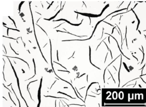
Figure 9. Grey cast iron or lamellar graphite iron (LGI) [16]
