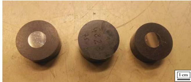
Figure 22. Samples mounted in a baquelite cylinder
