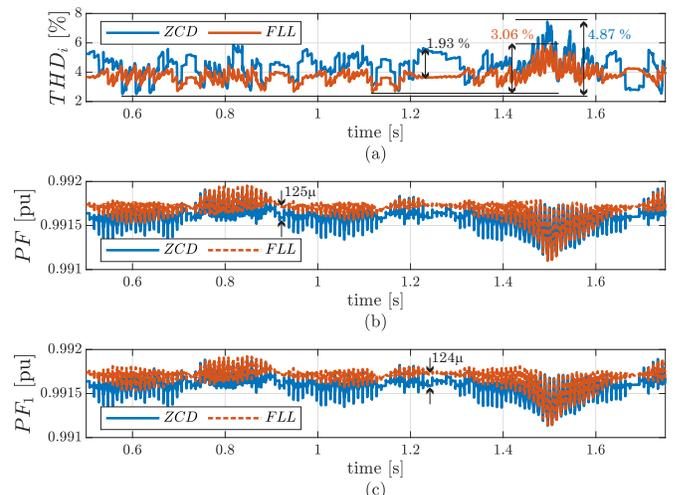
Fig. 8: Grid frequency variations with pure sinusoidal grid voltage. a)  $THD_i$ , b)  $PF$ , and c)  $PF_1$ .
