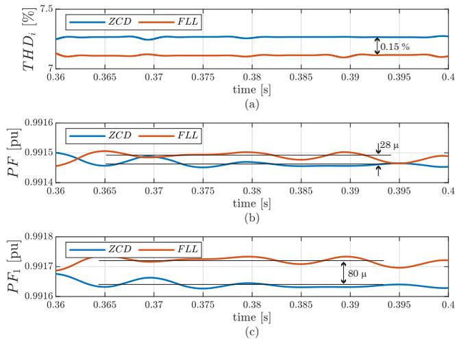
Fig. 6: Steady-state results with harmonically distorted grid voltages. a)  $THD_i$ , b)  $PF$ , and c)  $PF_1$ .
