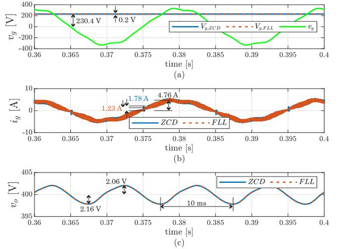
Fig. 5: Steady-state results with harmonically distorted grid voltages. a) grid voltage, b) grid current, and c) output voltage
