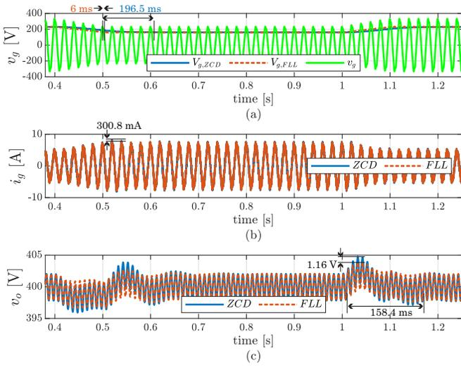
Fig. 9: Slow voltage dip with harmonically distorted grid voltage. a) grid voltage, b) grid current, and c) output voltage.
