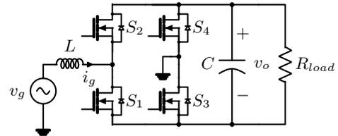
Fig. 1: Single-phase bridgeless totem-pole PFC.
