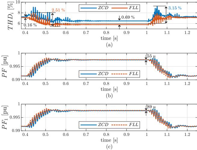
Fig. 10: Slow voltage dip with harmonically distorted grid voltage. a)  $THD_i$ , b)  $PF$ , and c)  $PF_1$ .
