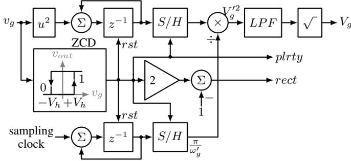
Fig. 3: Conventional implementation of the *polarity & rms calculation* block.
