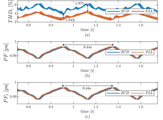
Fig. 12: Slow voltage variations with pure sinusoidal grid voltage. a)  $THD_i$ , b)  $PF$ , and c)  $PF_1$ .
