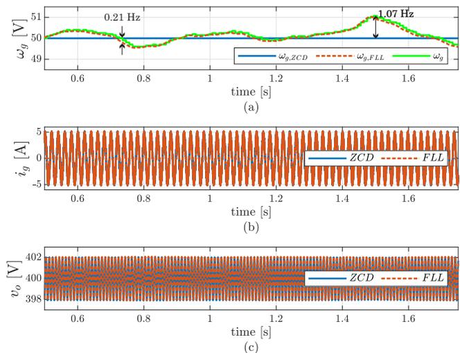
Fig. 7: Grid frequency variations with pure sinusoidal grid voltage. a) grid voltage, b) grid current, and c) output voltage.
