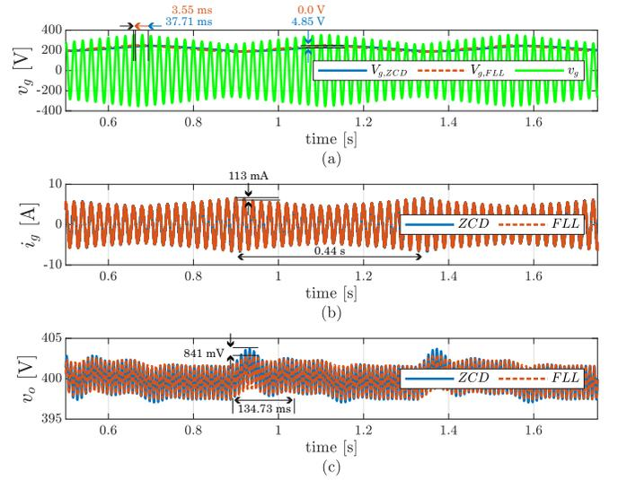
Fig. 11: Slow voltage variations with pure sinusoidal grid voltage. a) grid voltage, b) grid current, and c) output voltage.
