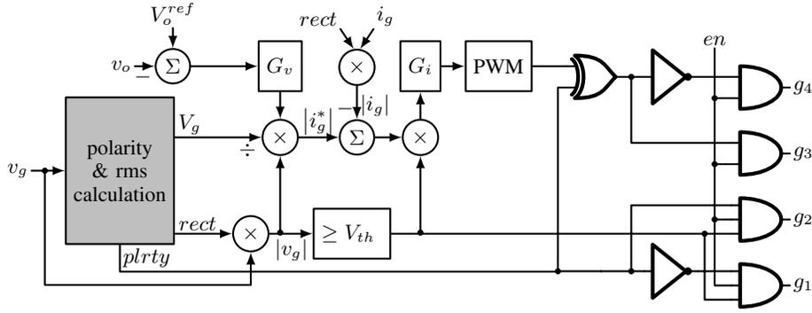
Fig. 2: Digital controller with rectified ac variables for the single-phase bridgeless TP PFC.
