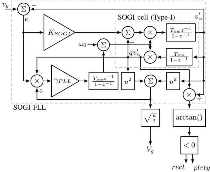
Fig. 4: Proposed implementation of the *polarity & rms calculation* block.
