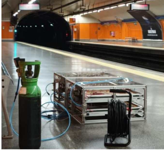
Figure 3.2: Muon Systems MWPCs prepared for the first tests performed in underground railway tunnels.
