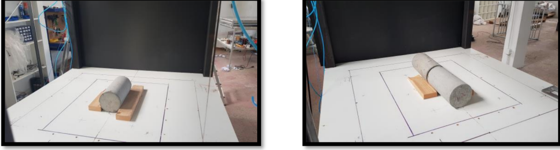
Figure 4.2: On the left, the scenario used to emulate an intact concrete structure. On the right, the scenario of the cracked concrete structure.
