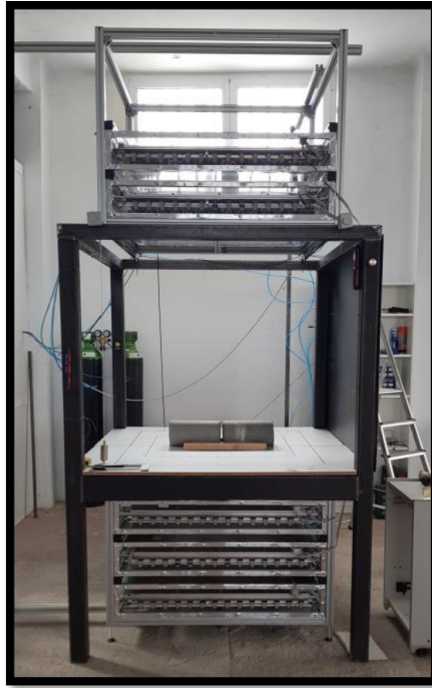
Figure 4.1: The MWPC detectors located in their structure with the concrete samples placed in between.
