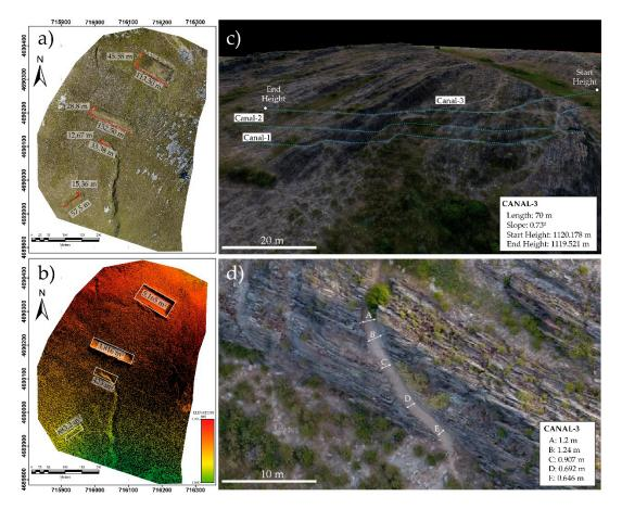
**Figure 7.** (**a**) Orthomosaic and (**b**) DSM from water reservoirs also called *maseras* (Model 5). 3D model of hydraulic infrastructure (Model 6). (**c**) Three supply canals excavated in slates. Water flow from right to left. Measurements of dimensions and characteristics of canal 3. (**d**) Differences in diameter measured in canal 3 along a curved section.
