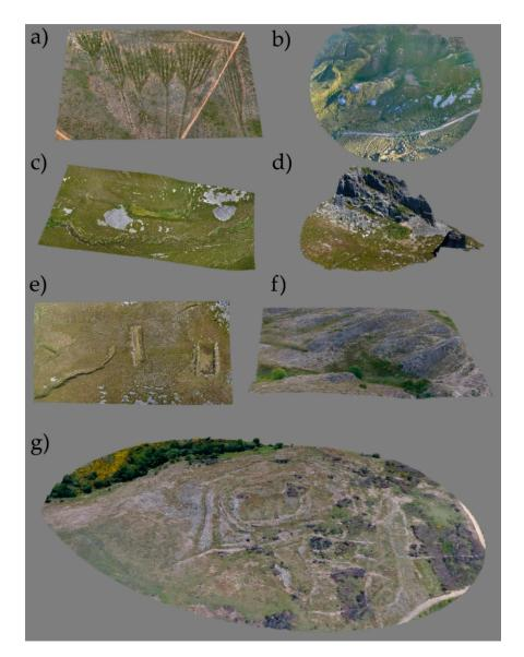
**Figure 8.** 3D texture models: (**a**) shallow open-cast mine (Model 1); (**b**) deep open-cast mine (Model 2); (**c**) tailing deposits (Model 3); (**d**) rock tunnel (Model 4); (**e**) stepped water reservoirs (Model 5); (**f**) supply canals (Model 6) and (**g**) mining camp (Model 7). Models available in Supplementary Materials (Figures S1–S7).
