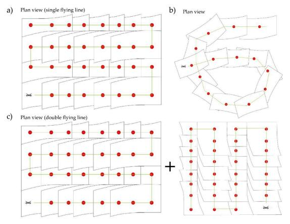
**Figure 5.** Flying modes implemented for mapping mining sites presented in this work. (**a**) Automatic flying mode and a single flying line: Model 1; (**b**) Manual flight: Model 3, 4 and 7; (**c**) automatic grid and double flying line: Models 2, 5 and 6. Red dots locate the image photocenters and black lines represent the image marks.
