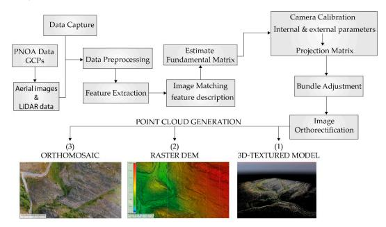
**Figure 3.** Structure from Motion (SfM) process of image implementation and derived data. Processing of images comprises computer vision feature extraction and image matching before the initialization of matrix estimations and camera parameters calibration necessary for the bundle adjustment. The final processes consist of the generation of dense point clouds from which a 3D-texture, a DEM and an image orthomosaic are obtained respectively.
