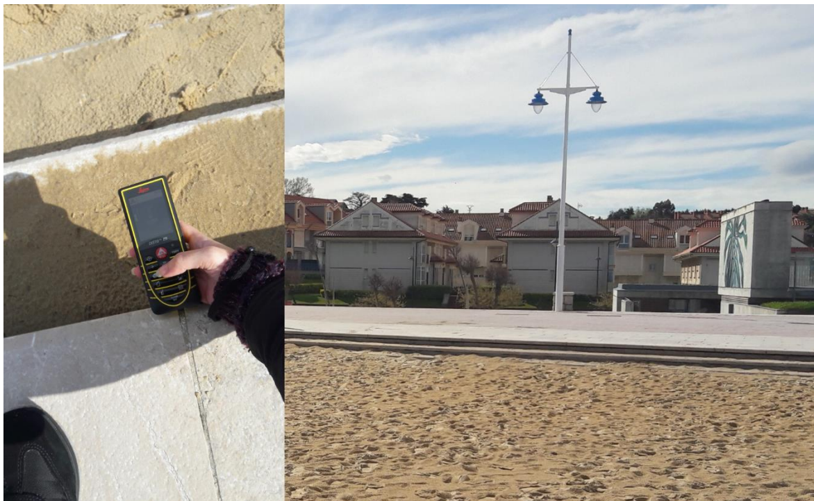
Figure 3.11 Example of profile definition (Somo P1). Left: Origin at the joint between the stone tiles of the upper stair at the entrance to the beach. Right: Orientation definition by the alignment of the streetlight and the ridge of the roof.
