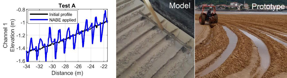
Figure 5.4 Ploughing. Left: Zoom of a profile of the ploughing performed in Channel 1. Centre: Picture of ploughing being conducted at the model at a reduced scale. Right: Example of ploughing at prototype scale at Laida beach (Source: Gainza et al., 2019).
