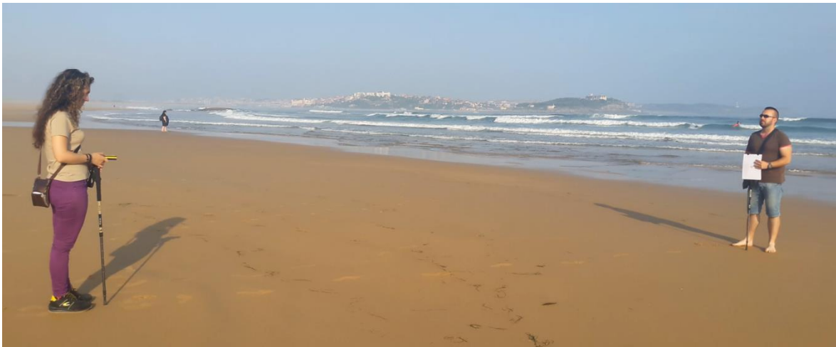
Figure 3.12 Measurement procedure for obtaining each profile point. On the left the surveyor S1 with the distancemeter device on the top of the walking stick, and at the right the other surveyor S2 with the target at the top of the walking stick. Both walking sticks were set to the same height.
