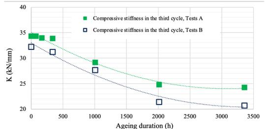
Fig. 6. Evolution of the compressive stiffness of the spacers as a function of ageing duration.
