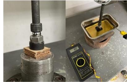
Fig. 1. Radial spacers under compressive loading in (a) type A tests and (b) type B tests, immersed in paraffinic oil.
