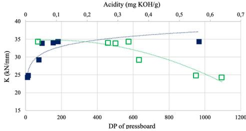
Fig. 7. Compressive stiffness of the high-density pressboard as a function of the DP and the acidity.
