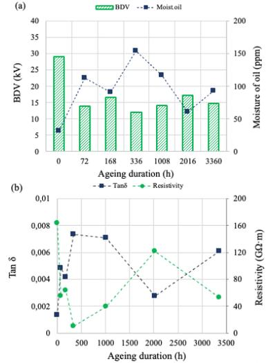
Fig. 3. (a) BDV and moisture content of the dielectric oil, (b) dissipation factor ( $\tan \delta$ ) and resistivity, as a function of thermal ageing duration.
