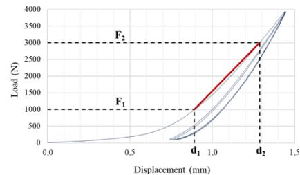
Fig. 2. Process for obtaining the compressive stiffness of the radial spacers from the force-displacement curves.
