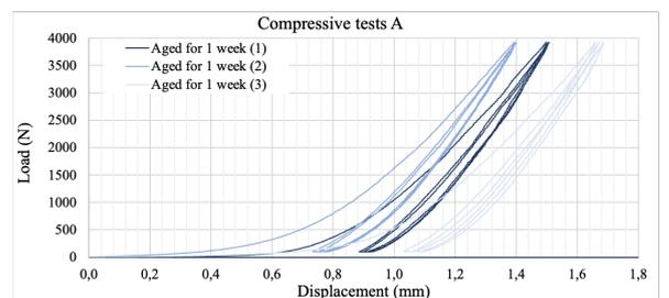
Fig. 5. Compressive Test A over the pressboard prism for an ageing duration of 1 week.
