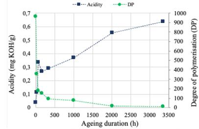
Fig. 4. Acidity in the oil and DP of the pressboard as a function of thermal ageing duration.
