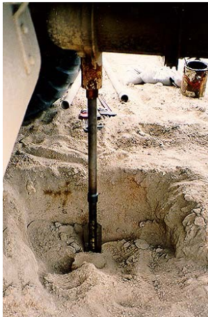
Figura 1.6: Ensayo in situ "Vane Shear Test"
