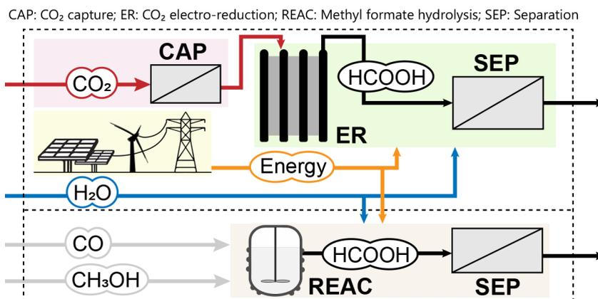
**Figure 2.** Cradle-to-gate system boundaries for CO<sub>2</sub>ER and fossil routes of HCOOH production. The functional unit for the case study is defined as producing 1 kg of commercial HCOOH.
