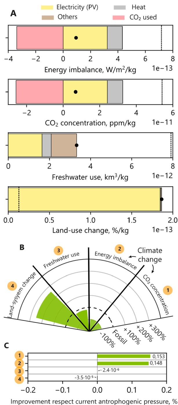
**Figure 5.** (A) Environmental performance in selected PB indicators for producing 1 kg of HCOOH in CO<sub>2</sub>ER route (best-case scenario). The fossil route is noted as a dotted line. (B) The ratio between the environmental burdens for the production of HCOOH by CO<sub>2</sub>ER and fossil routes. (C) Change in the level of transgression from anthropogenic pressures when HCOOH production changes from the fossil to the CO<sub>2</sub>ER route.
