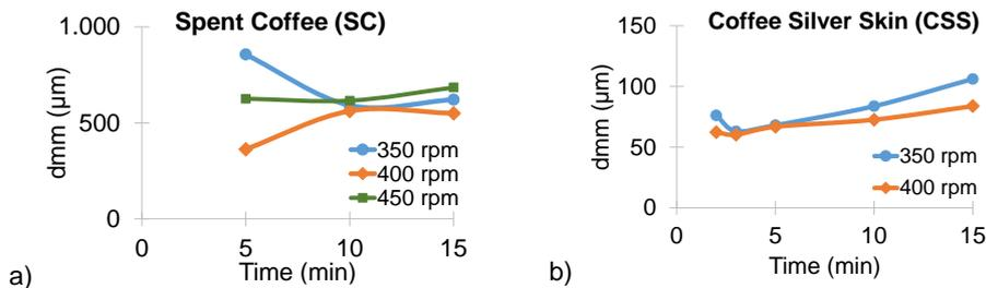
Figure 1. Influence of grinding time and rotational speed variables on the average particle size: a) SC, b) CSS
