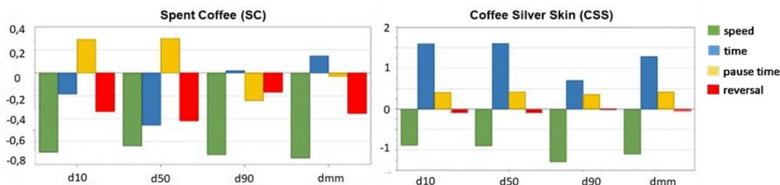
Figure 3. Graph of coefficients for  $d_{10}$ ,  $d_{50}$ ,  $d_{90}$  and  $d_{mm}$  for SC and CSS (rotational speed, grinding time, pause time, reversal of direction).
