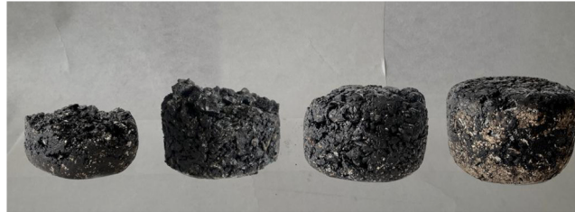
Fig. 16. Final condition of samples sometimes tested in Cantabro. From left to right: Ref Spain, Ref U.S. Institute, EM1 and EM2.
