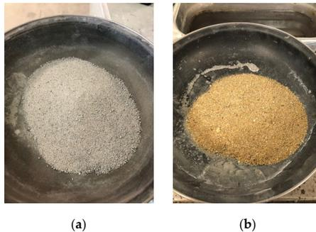
Figure 3.2. Used foundry (a) sand and silica sand (b).
