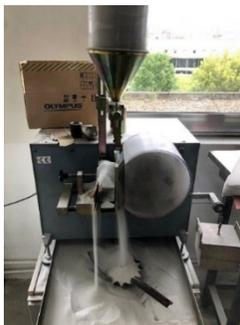
Figure 3.4. Set up of the abrasion wear resistance test.
