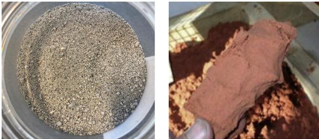
Figure 2.2. Green foundry sand (left) and Chemical foundry sand. Source: [65].
