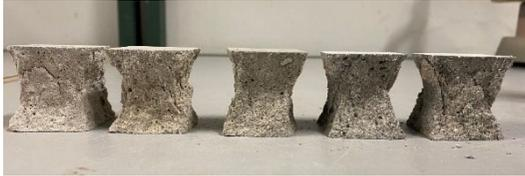
Figure 3.16. Mortar specimens with UFS, from 0 to 100%.
