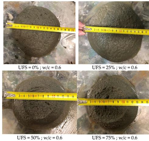
Figure 3.8. Mortar workability: slump table test results. Comparative example for a fixed w/c ratio.
