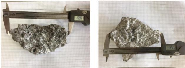
Figure 4.2. Untreated siderurgical aggregates.
