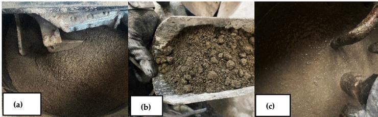
Figure 5.2. Mix procedure: dry mix of the aggregates (a); addition of first part of mixing water (b); settling of the SCC mix by 3 min (c).
