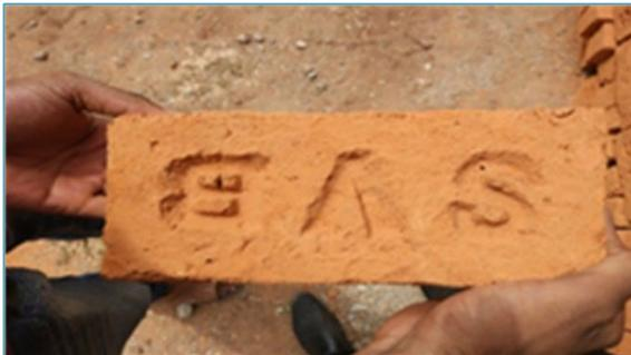
Figure 2.6. Bricks manufactured with UFS. Source: [91].
