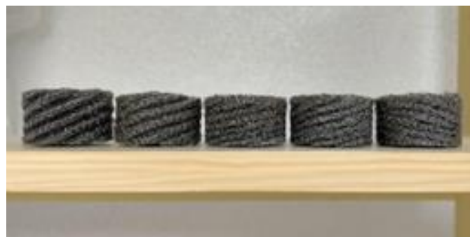
Figure 6. Five isolator models with different relative density.
