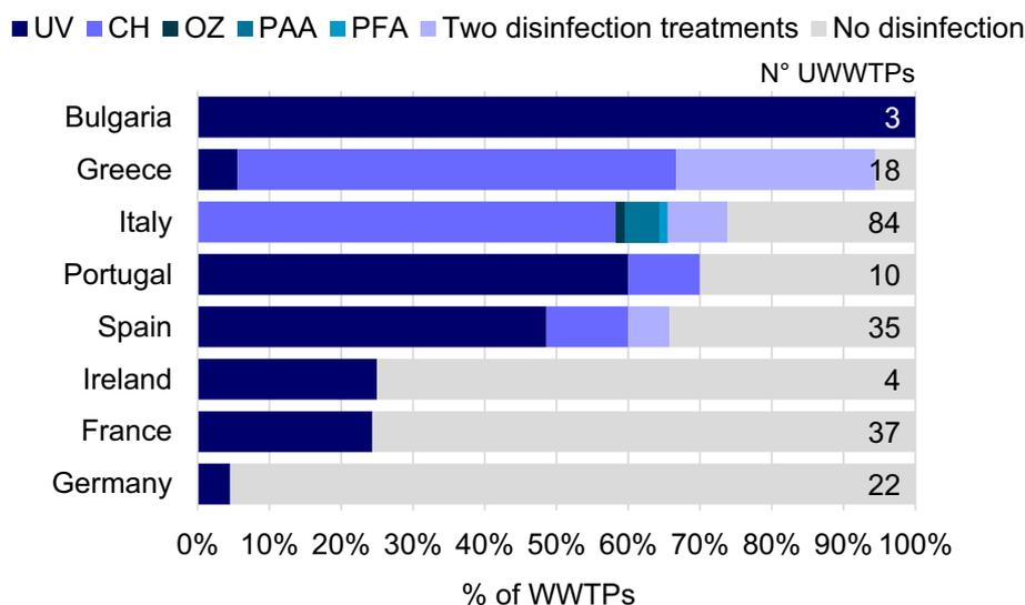
**Fig. 7.** Percentage distribution of selected UWWTPs according to the disinfection treatments applied to the effluent and number of treatment facilities in each country. The disinfection treatments considered are ultraviolet (UV), chlorination (CH), ozonation (OZ), peracetic acid (PAA) and performic acid (PFA).
