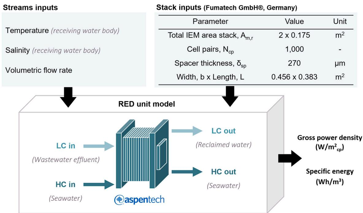
Fig. 2. Simulation diagram adapted to the parameters analysed in the study.
