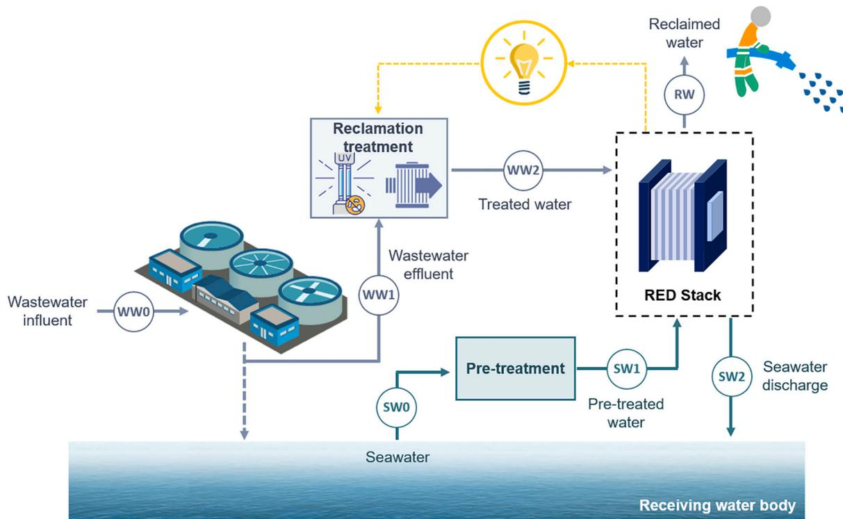
Fig. 1. Water reclamation process powered by salinity gradient energy overall flow diagram. Adapted from Gómez-Coma et al. (2020).
