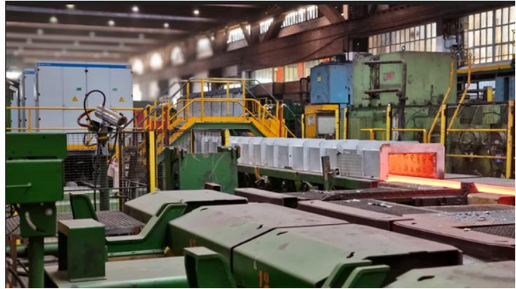
Figure 1.2: Billet exiting GSW's induction furnace.
