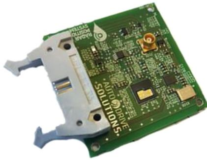
**FIGURE 6** Radar sensor that has been developed to read the railway track profile.
