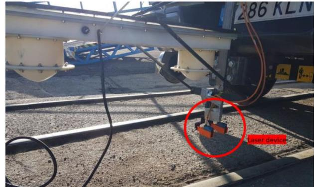
**FIGURE 14** (Right) Location of the laser profilometer at the drain.
