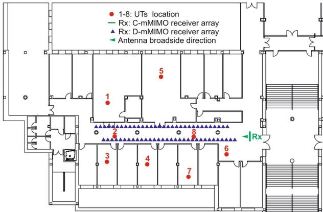
**Fig. 1.** Top view of the indoor environment (measurements in the 3.3-3.7 GHz frequency band).
