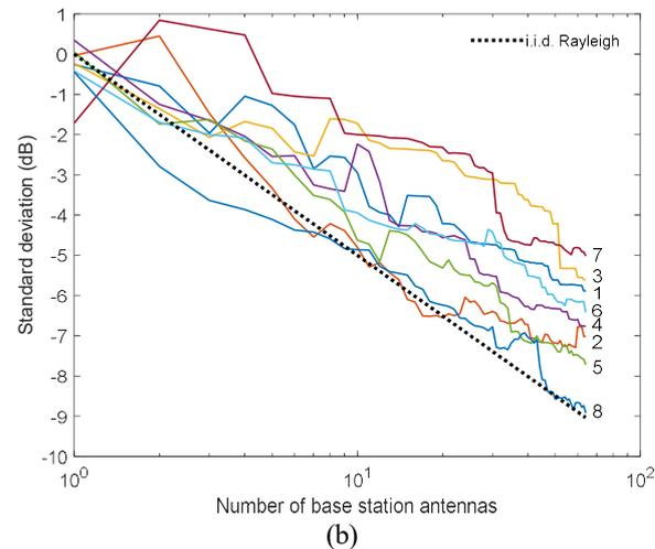
**Fig. 2.** Standard deviation of the channel gain for the 8 UTs in the 3.5 GHz band. (a) C-mMIMO. (b) D-mMIMO.
