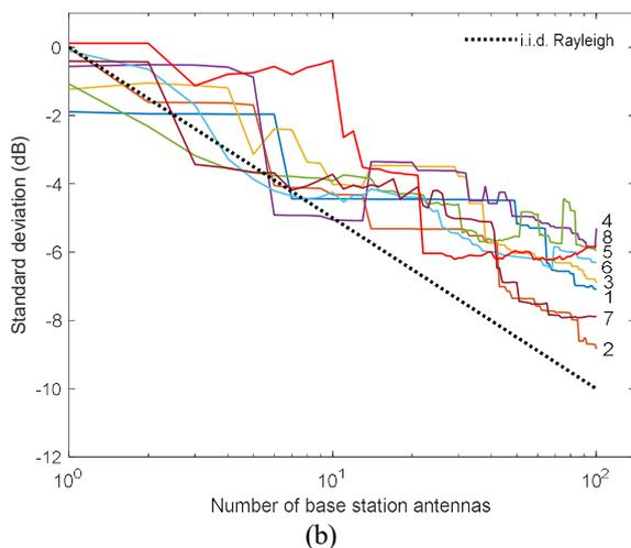
Fig. 4. Standard deviation of the channel gain for the 8 UTs in the 26 GHz band. (a) C-mMIMO. (b) D-mMIMO.
