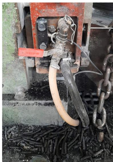
Fig. 19. Carbonized debris disperse around the die box bench form the delaminated phosphate layer waste due to the die overheating (Test 2b).
