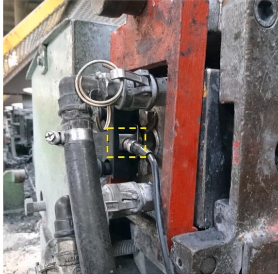
**Fig. 4.** Picture of the AE sensor positioned in contact with the die box using a magnetic holder.
