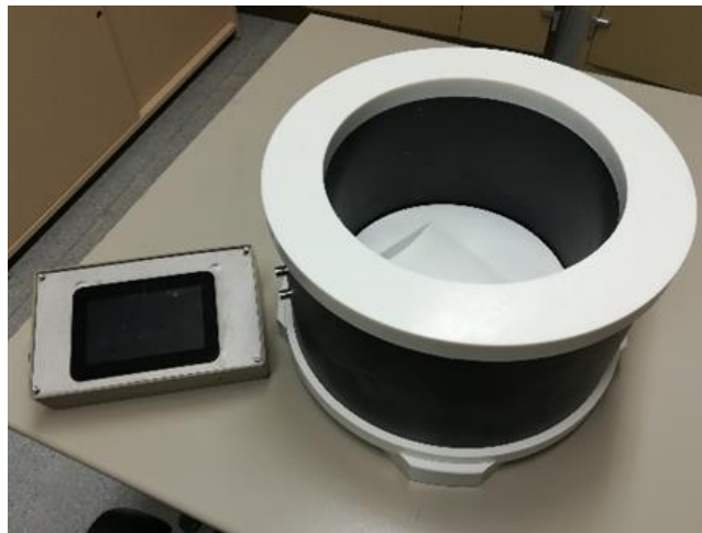
Fig. 8. Inductive equipment SmartFibreC® for the quantification of the amount and orientation of steel fibres in hardened concrete.
