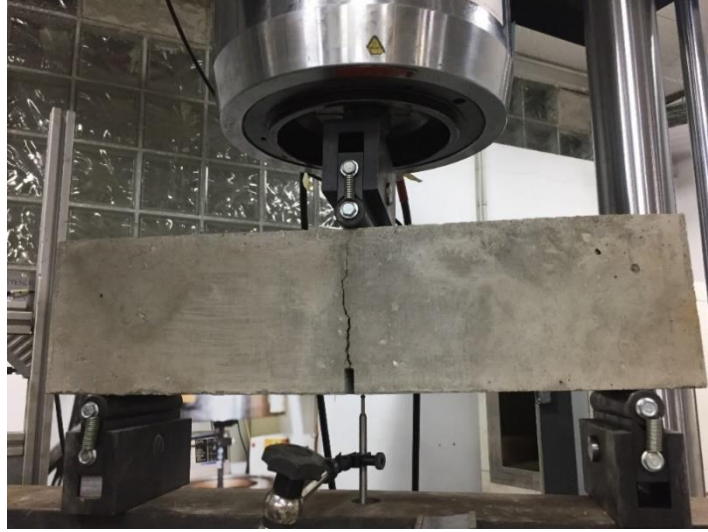
Fig. 4. Flexural tensile strength test of the fibre reinforced concrete.
