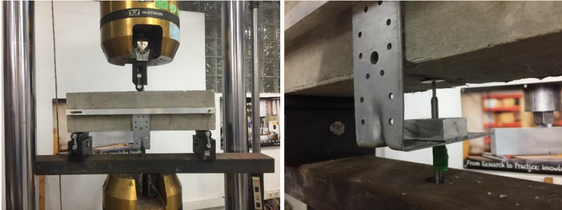
Fig. 22. Flexural tensile strength test (left) and measurement of vertical displacement with a LVDT (right).
