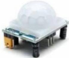
This motion sensor module uses the LHI778 Passive Infrared Sensor and the BISS0001 IC to control how motion is detected.
