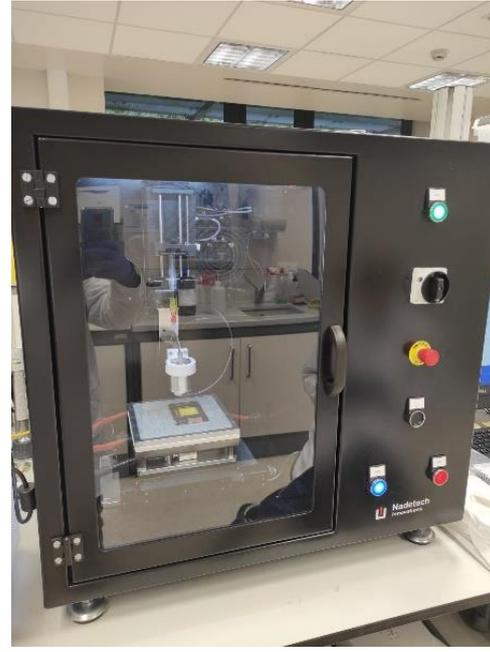
Figura 7 ND-SP Mini Ultrasonic Spray Coater Nadetech Innovations®.
