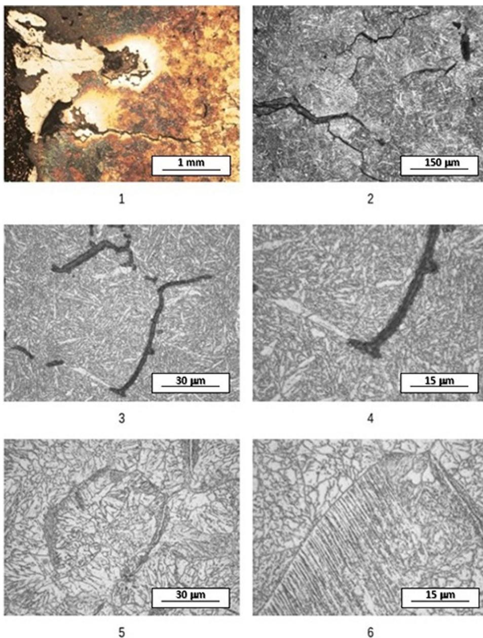
needle-like shape growth of bainite can be observed in this same microstructural area arranged in parallel bands and following a preferential orientation within the previous austenitic grain from its boundary (Fig. 10(6),  $\times 1000$ ). In this part of the piece, the microhardness determinations made with an applied load of 100 g yield values that range between 175.0 HVN and 199.3 HVN, with an average value of 187.8 HVN.
