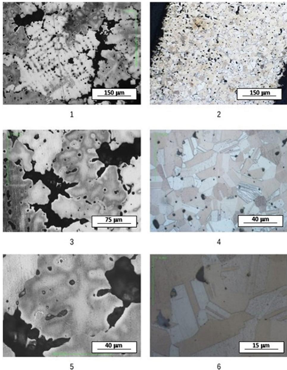
dispersed lead globules, in line with the low lead content of alloys. The porosity and the oxide inclusions suggest that the temperature of the crucible may have been too high and that an open mold was possibly used in the casting [33].
