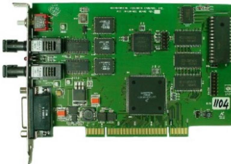
Figure 21: The ARC-66 PCI Interface Board
