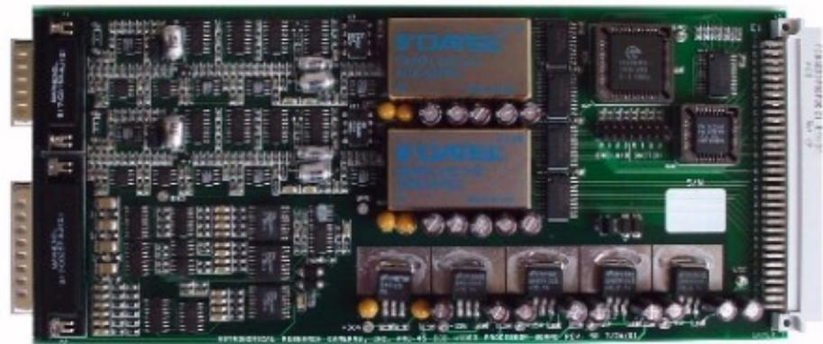
(c) The ARC-45 Two Channel CCD Video Board.
