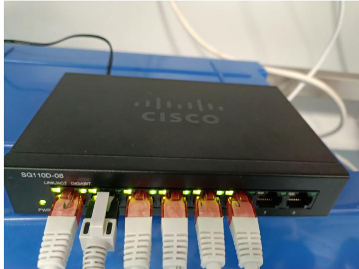
(a) Switch Network device connected to the Ethernet network.
