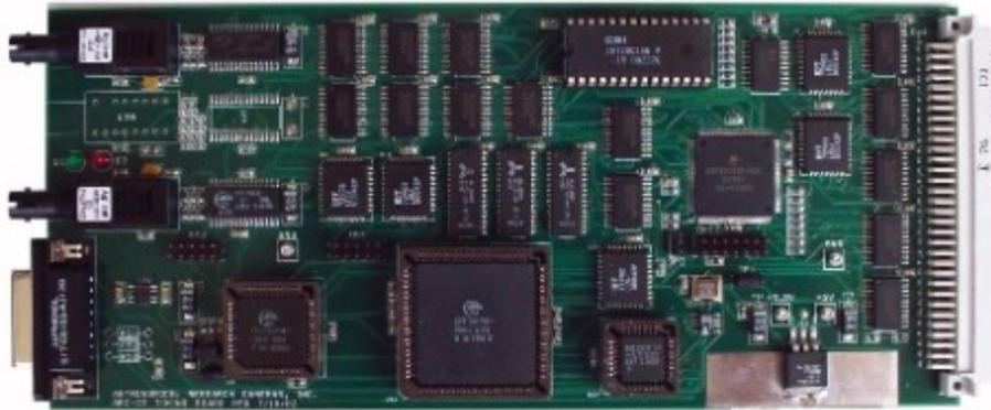
(a) The ARC-22 250 Mhz Fiber Optic Timing Board.
