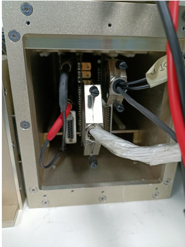
Figure 20: Image of the 6-Slot Closed Housing System with the corresponding installed boards, from left to right, the Fiber Optic Timing board, CCD Clock Driver and CCD Video board.
