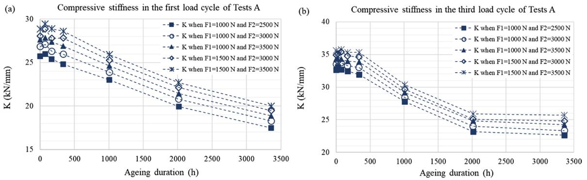
**Fig. 12** Different values of the compressive stiffness of high-density pressboard,  $K_{pressboard}$ , as a function of the ageing duration in **a** the first load and **b** the third loading cycle of Tests A
