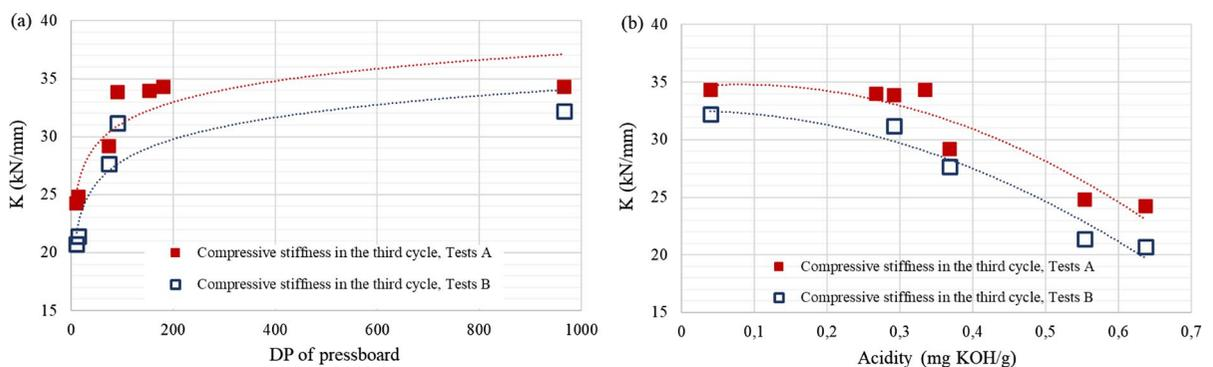
**Fig. 15** **a** Relationship between the compressive stiffness of the high-density pressboard and the degree of polymerisation, DP; **b** Relationship between the compressive stiffness of the high-density pressboard and the acidity
