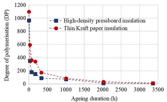
**Fig. 8** Reduction of the DP as a function of the duration of thermal ageing
