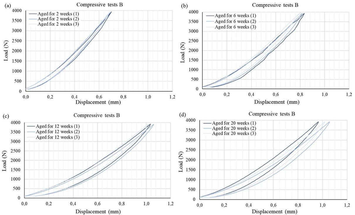
**Fig. 11** Load–displacement curves for the third cycle in compressive tests B, for ageing durations of **a** 2 weeks, **b** 6 weeks, **c** 12 weeks and **d** 20 weeks
