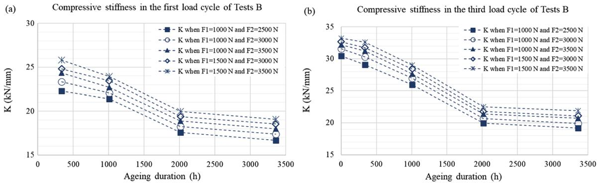
**Fig. 13** Different values of the compressive stiffness of high-density pressboard,  $K_{pressboard}$ , as a function of the ageing duration in **a** the first load and **b** the third loading cycle of Tests B
