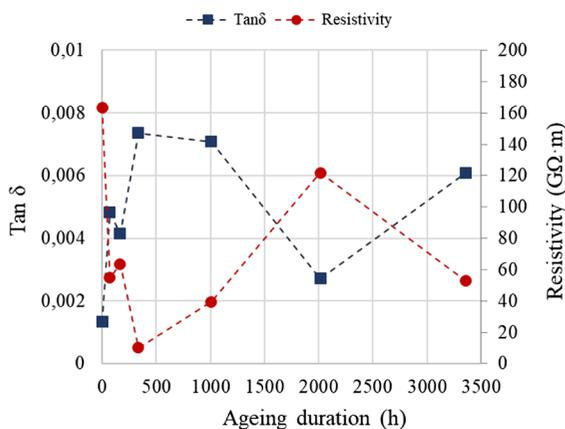
**Fig. 6** Dielectric dissipation factor ( $\tan \delta$ ) and resistivity as a function of the duration of thermal ageing
