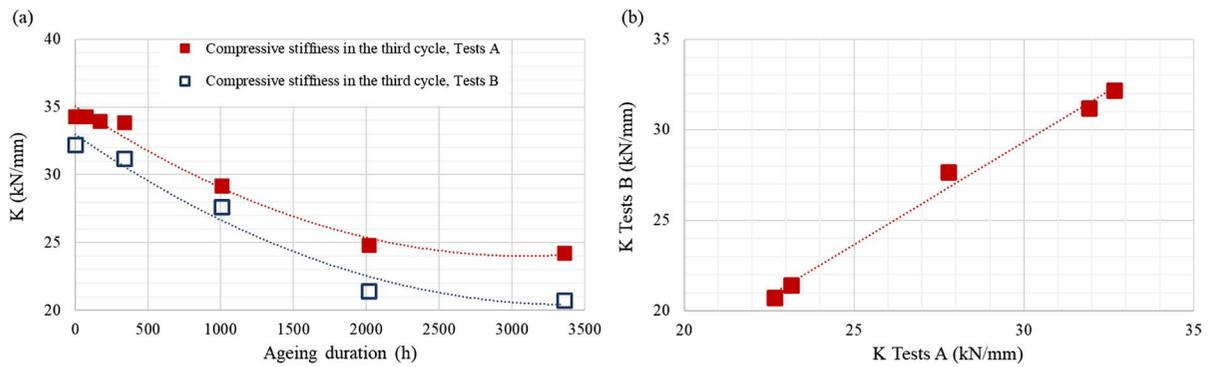
**Fig. 14** **a** Evolution of the compressive stiffness of the high-density pressboard as a function of ageing duration, for both tests A and B; **b** Relationship between the compressive stiffnesses in the third loading cycle for tests A and B
