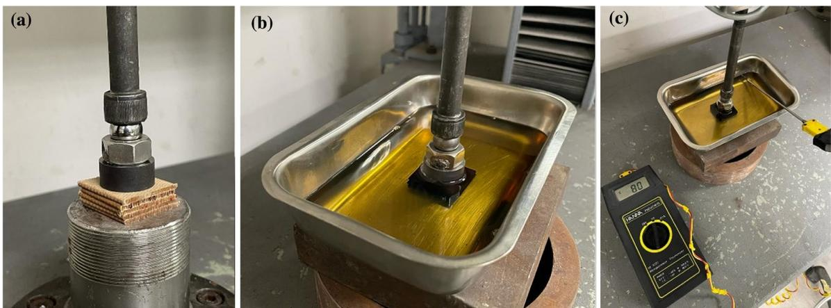
**Fig. 3** Prism made of high-density pressboard samples being subjected to compressive tests **a** type A, in open-air, and **b** type B, immersed in dielectric oil
