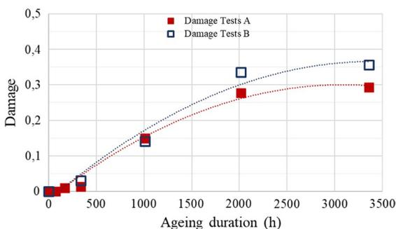
**Fig. 16** Evolution of the damage,  $D$ , as a function of ageing duration
