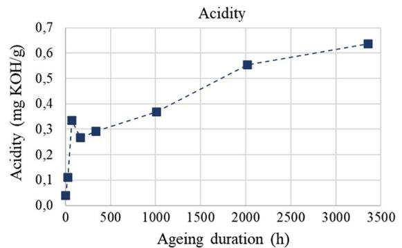
**Fig. 7** Acidity in the oil as a function of the duration of thermal ageing
