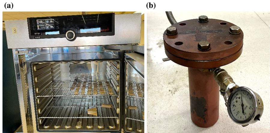
of the drying process, meaning that a higher reduction in moisture content was not possible with the laboratory equipment available. The paraffinic oil was also vacuum-dried at 105 °C for 3 h, to reduce its initial moisture content up to 32.1 ppm. After drying, the pressboard was immersed in oil for its impregnation, at 60 °C during 24 h.
