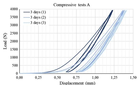
**Fig. 9** Load–displacement curve for compressive Test A over the pressboard prism, with three cycles of loading–unloading, for an ageing duration of 3 days
