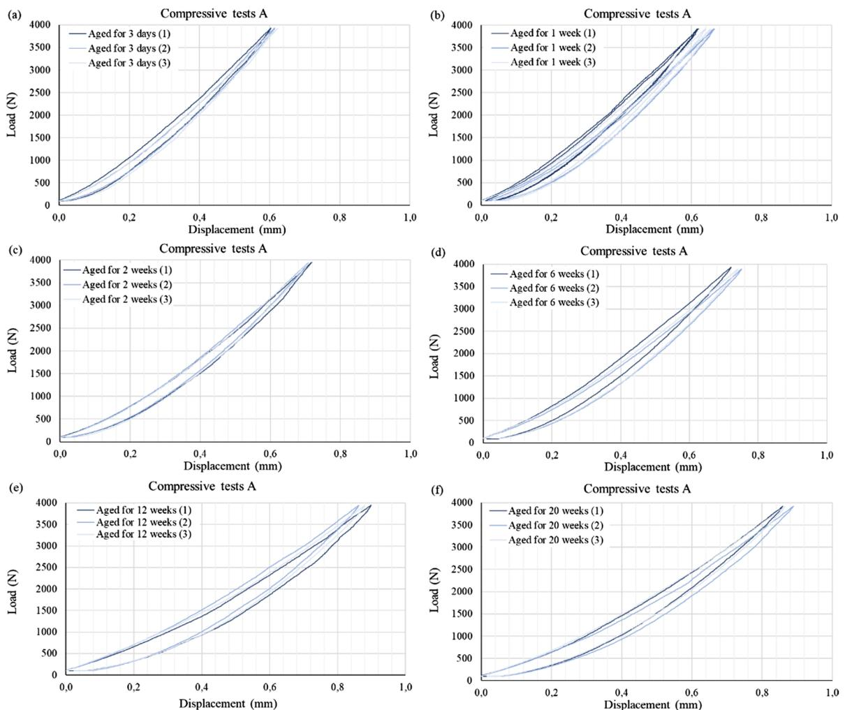
**Fig. 10** Load–displacement curves for the third cycle in compressive tests A, for ageing durations of **a** 3 days, **b**) 1 week, **c** 2 weeks, **d** 6 weeks, **e** 12 weeks and **f** 20 weeks
