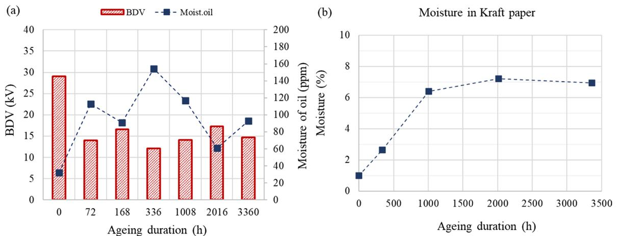
**Fig. 5** **a** AC breakdown voltage (BDV) and moisture content of the dielectric oil, **b** Moisture content in the Kraft paper insulation, as a function of the duration of thermal ageing
