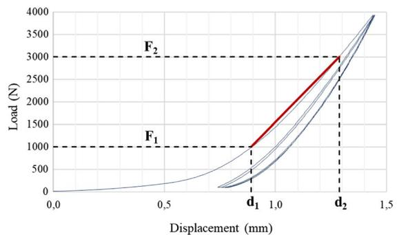
**Fig. 4** Process for obtaining the compressive stiffness of the high-density pressboard, in this case for the first compressive cycle, from the force–displacement curves
