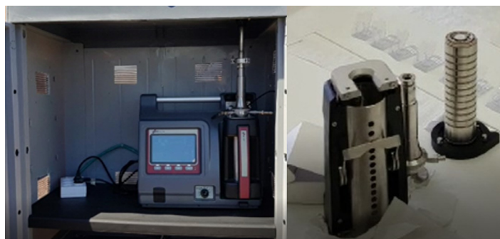
Fig. 2. Electrical low-pressure impactor (ELPI®+) with 14 channels vertical sampling line.
