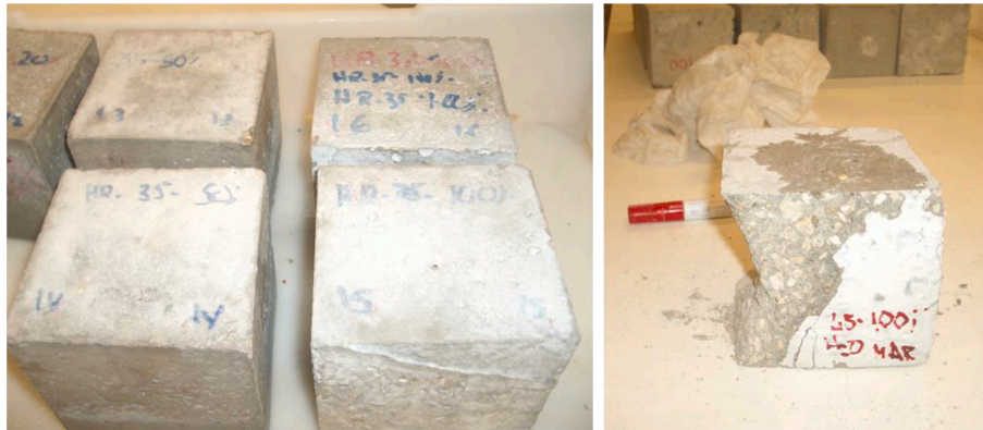
Fig. 13. Appearance of specimens after completion of the marine-water moist/dry test.
