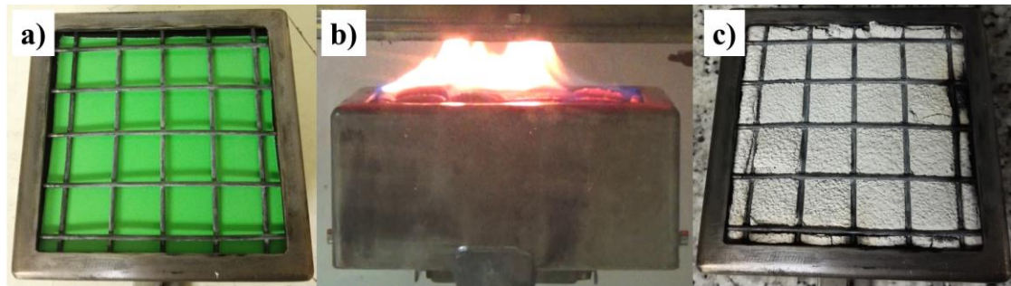
Figure 1. Sheath sample tested in cone calorimeter: a) before, b) during and c) after.
