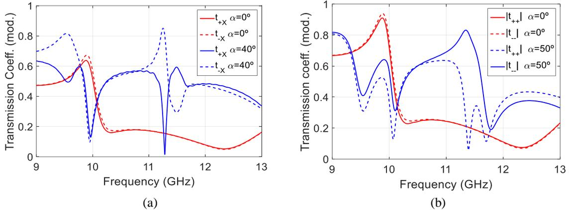
Fig. 5. Linear to circular (a) and circular (b) transmission coefficients of the mutual twist rosette structure with  $\phi = 30^\circ$  arranged in a sawtooth profile distribution
