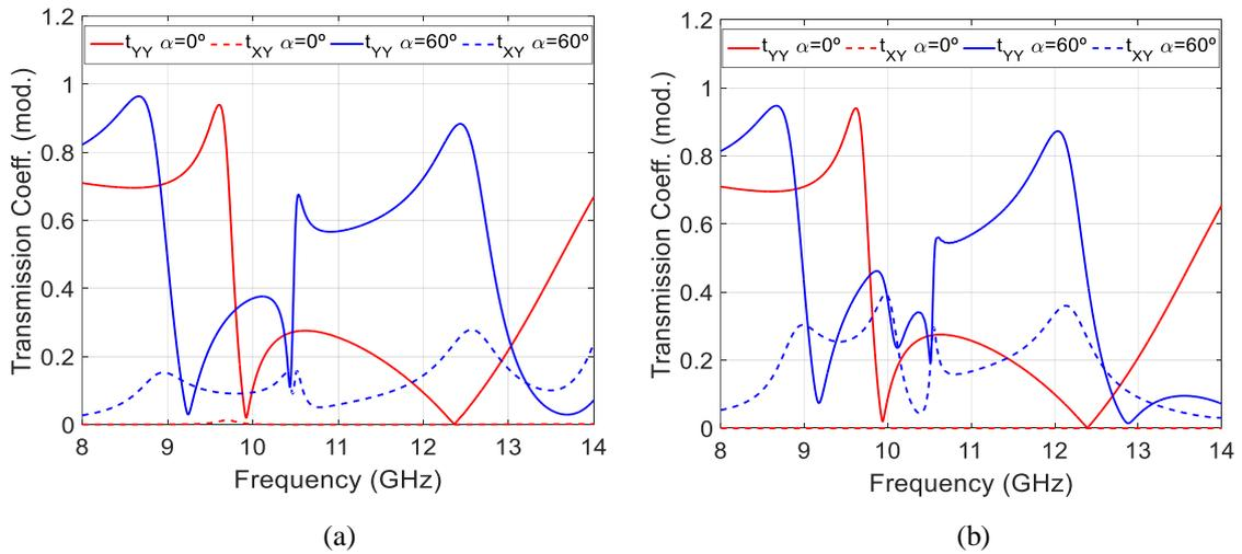
Fig. 4. Linear co-polar and cross-polar transmission coefficients with  $\phi = 0^\circ$  and  $\alpha = 0^\circ$  (red line),  $60^\circ$  (blue line) (a) sawtooth and (b) zigzag profile.
