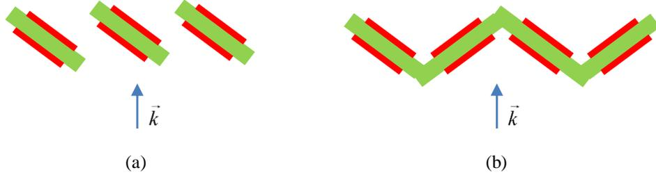
Fig. 1. Profile view (a) Sawtooth profile, (b) Zigzag profile. (Red: metallization/Green: substrate).
