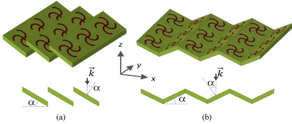
Fig. 3. Mutual twist rosettes distributed in a (a) Sawtooth profile, (b) Zigzag profile.
