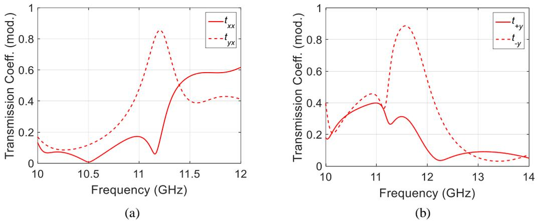
Fig. 6 Linear (a) and linear to circular (b) transmission coefficients of the mutual twist rosette structure with  $\phi = 30^\circ$  arranged in a zigzag profile with  $\alpha = 60^\circ$ .
